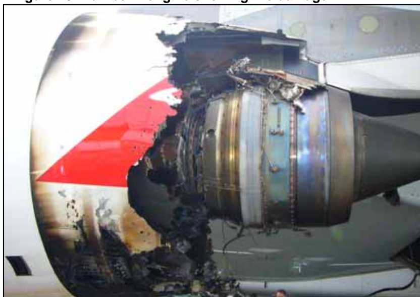
Figure 13: Number 2 engine showing fire damage
