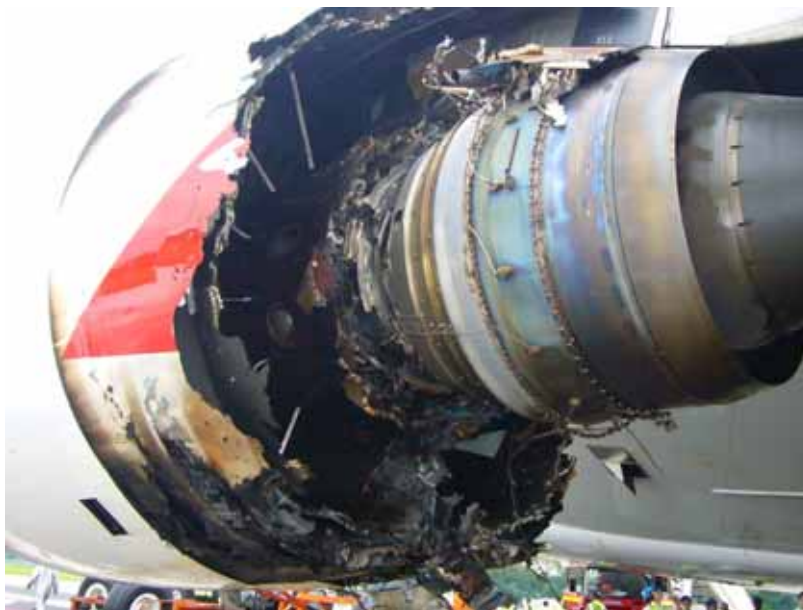
Figure 7: Damage to the No 2 engine
