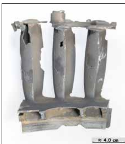
Figure 16: Portion of LP turbine first stage nozzle guide vanes that was recovered from Batam Island, Indonesia
